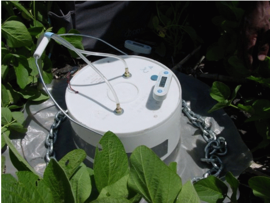
Example of temporary/portable chamber used by Parkin. Chamber has an attached polyethylene skirt held in place on the soil surface with a length of chain. As shown, the chamber is monitoring soil CO 2 flux by recirculating gas through an infrared analyzer. Gas samples can be withdrawn through septum in top of chamber for N 2 and CH 4 analyses.
